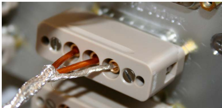
Figure – Actuator cable plugged on the feedthrough
