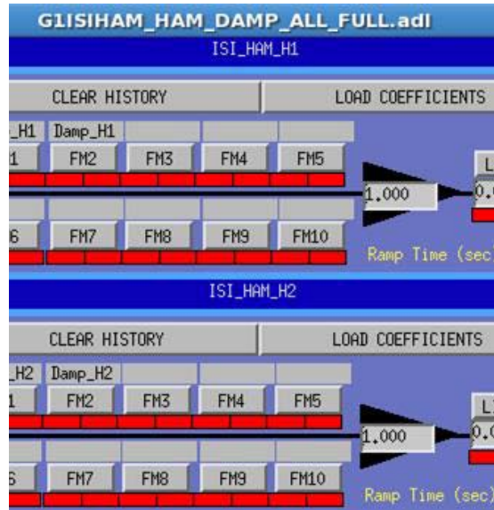
Figure – State of the damp MEDM screen- All gains must be set to 1!
