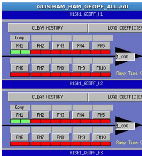
Figure – State of the Geophone readout MEDM screen: compensation filters need to be ON!
