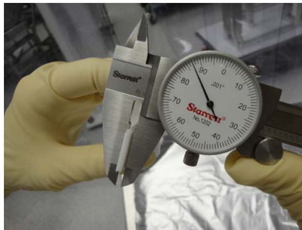
Figure - Stack of Teflon shims being measured for gap check of actuators.
