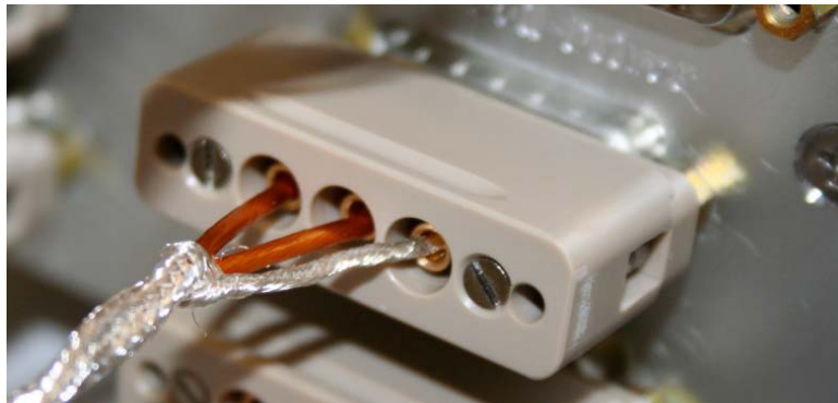
Figure – Actuator cable plugged on the feedthrough
