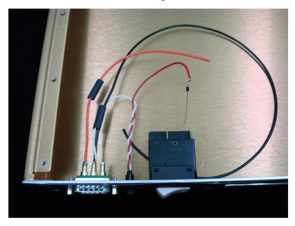
A current limiting diode (Digikey p/n 610-1N5314) cathode lead (the lead on the striped end of the diode body) is soldered onto the end of the anode (red) wire of the LED. Now refer to photo number 2. The other lead of the diode is then soldered to a 13" length of orange, 18AWG wire as shown in the photo. Shrink tubing is then used to hold the body of the diode and the LED lead securely to the orange wire.
