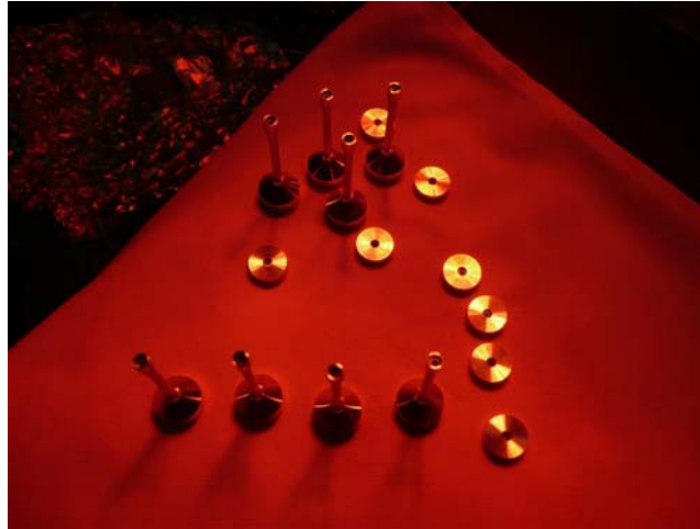
Figure 6.10 Glueing steel rings into the magnet flags
