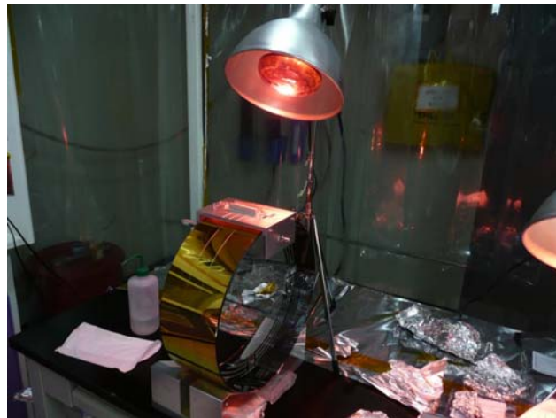
Adhesive curing on side 1
