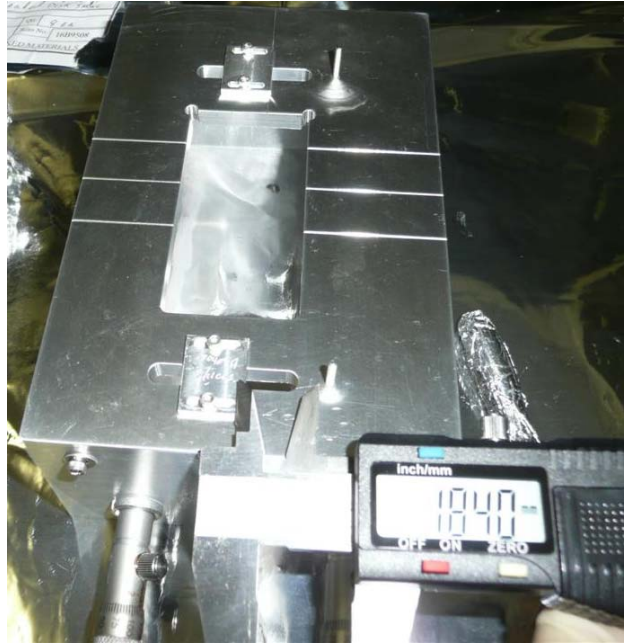
Figure 6.4 Setting prism bonding jig for side 2
