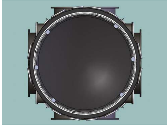
All four support ring sections installed
