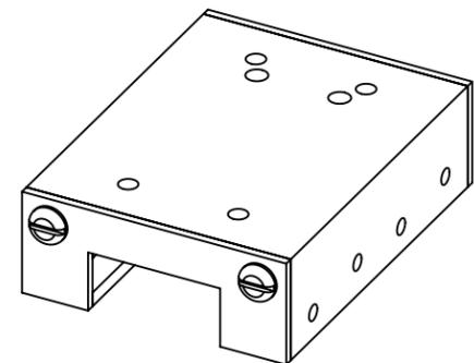
D1001945 aLIGO TMS DEL-TRON RS-1-1 VERTICAL CARRIAGE, PART PDM REV: X-007, DRAWING PDM REV: X-013
