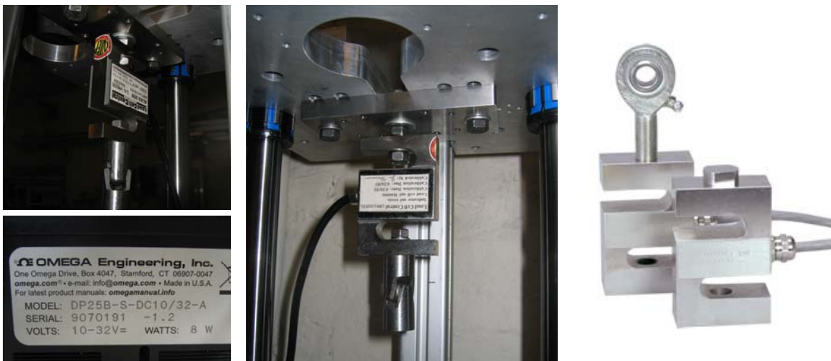
Figure 9: Load cell detail, XLS2-250 with meter
