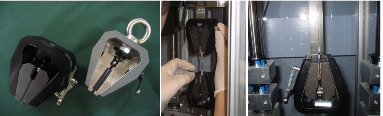
Figure 11: Wedge action grips, GF-11 by Lloyd Instruments
