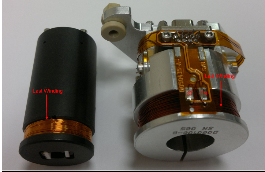
Figure 4c Coil winding sense of BOSEM compared to AOSEM
