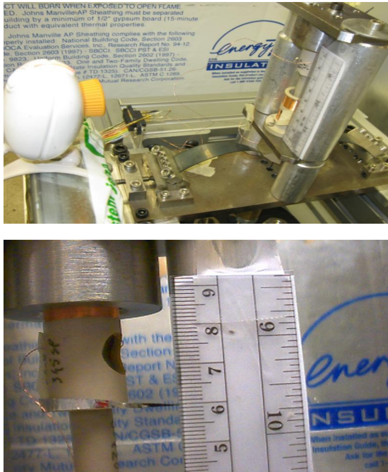
Figure 4.7: Proceedings adopted for the LVDTs calibration. The fixed camera (left on the top photo) stares at a stationary ruler and at a needle attached to the moving part of the GAS spring.
