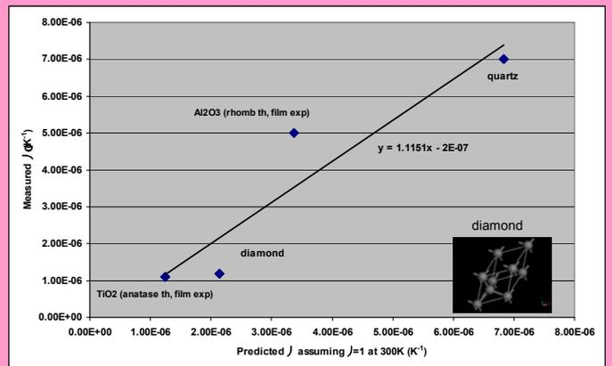
CASTEP Density Functional Theory calculation of CTE using computed values of C, B and the expression  $\alpha = gC/3B$  for Gruneisen parameter  $g=1$ .
