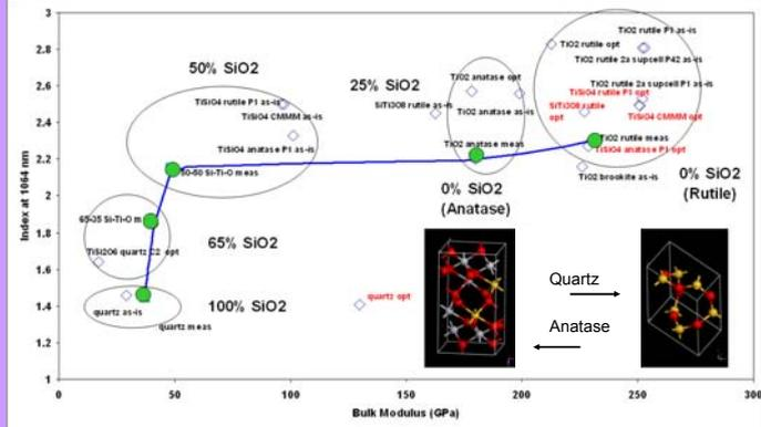
CASTEP Density Functional Theory calculation showing that when  $\text{TiO}_2$  rutile and anatase phases are doped with  $\text{SiO}_2$ , there is a plateau in the refractive index for a broad range of bulk moduli. Green points are experimental data, all else is a DFT prediction. Noting (\*\*), coating thermal noise could be minimized in  $\text{TiO}_2$  by  $\text{SiO}_2$  doping.
