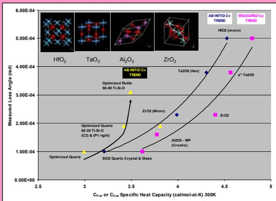
CASTEP Density Functional Theory calculation showing a trend with specific (atomic) heat capacity, with measured loss angle. The magenta data uses experimental values of the heat capacity  $C_p$ , demonstrating a reasonable prediction of that property as well. Comparing the predicted *ab initio*  $C_v$  (blue and yellow).
