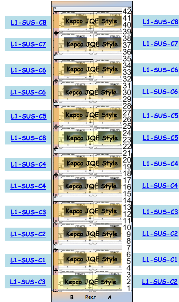
L1-VDC-C1 Power Rack
