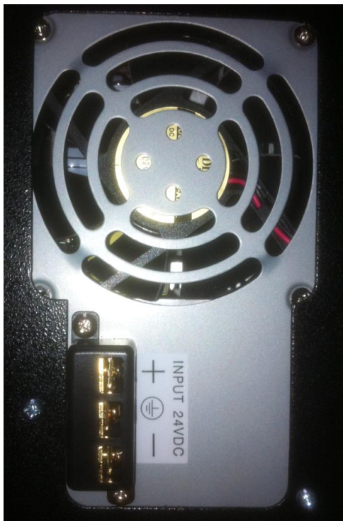
New 24VDC Power Supply
