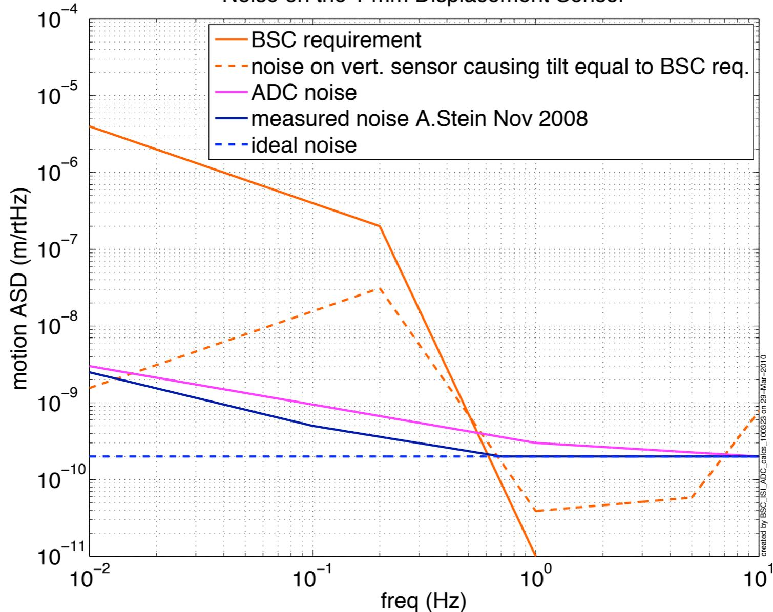
1. Measured noise at low freq is from thermal drift of test rig.
