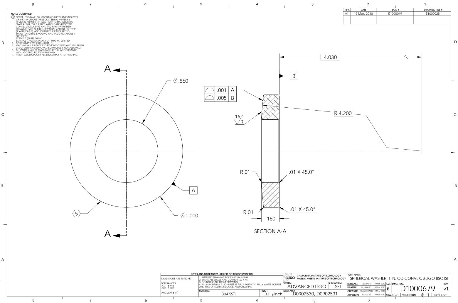
aligo BSC ISI, PART PDM REV: X-002, DRAWING PDM REV: X-002 1 in OD Convex D1000679 Spherical Washer,
