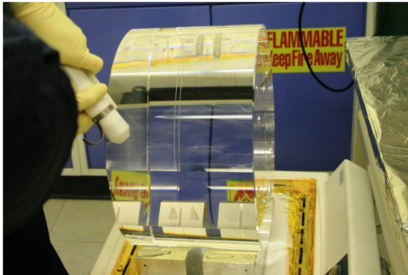
Figure 8 Drying the PUM with Nitrogen gas after cleaning
