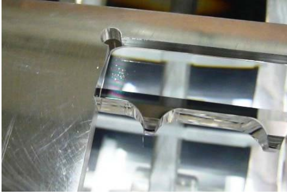
Figure 30 A few small bubbles and fringes visible shortly after bonding between ear 42 and test mass
