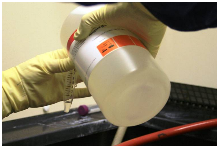
Figure 7 Making Bonding Solution using Sigma-Aldrich Sodium Silicate Solution
