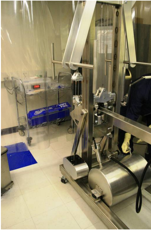
Figure 4 Ergo arm with pressure gauge receiver box in background
