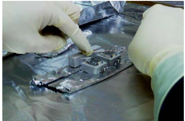
Figure 2 Applying vac-seal to prism base using a copper wire
