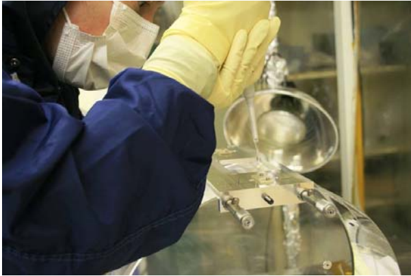
Figure 10 Pipetting bonding solution onto optic surface
