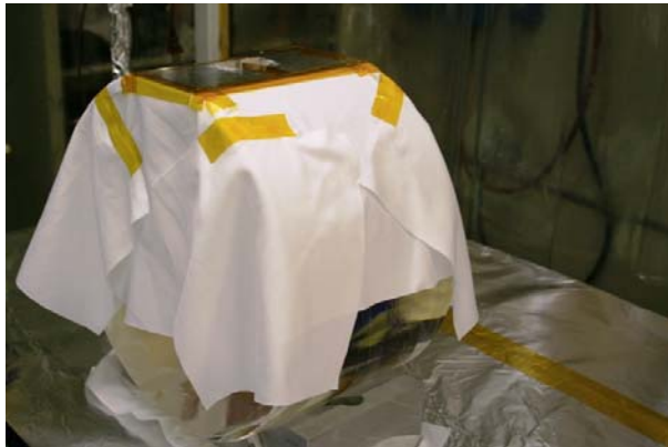
Figure 26 Protecting the test mass prior to removing old ears
