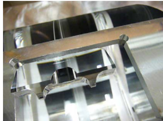
Figure 13 Ear 46 in place immediately after bonding with small bubbles visible
