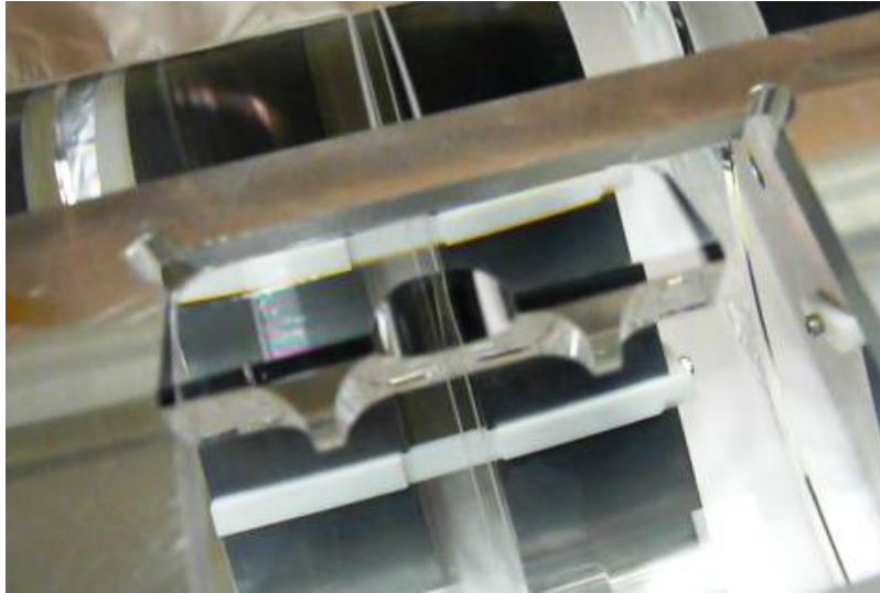
Figure 20 A few bubbles and fringes visible shortly after bonding between ear 51 and PUM
