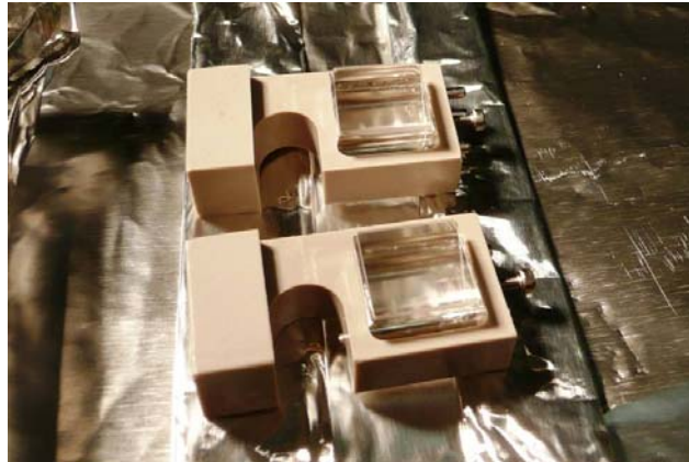
Figure 3 Prism and prism shims curing post-gluing under infra-red light
