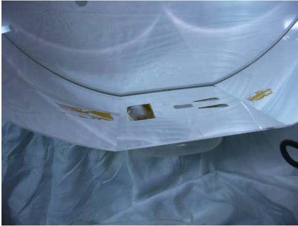
Figure 32 Slight haze in the bond on side 2 of the PUM
