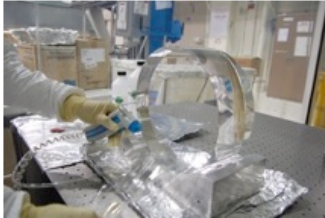
Figure 6: Keep a steady stream of nitrogen while peeling.
