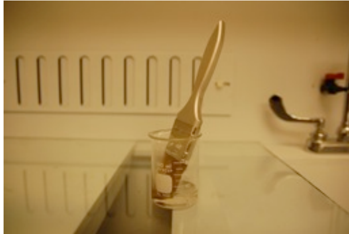
Figure 1: Small beaker with FC solvent and a PEEK/aluminum brush.
