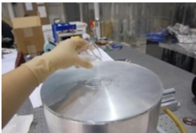
Figure 3: Pouring FC onto horizontal optic
