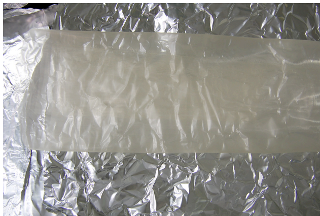
Figure 3: Roll of PEEK mesh on aluminum foil
