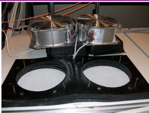
Gaskets in place showing "chimney"
