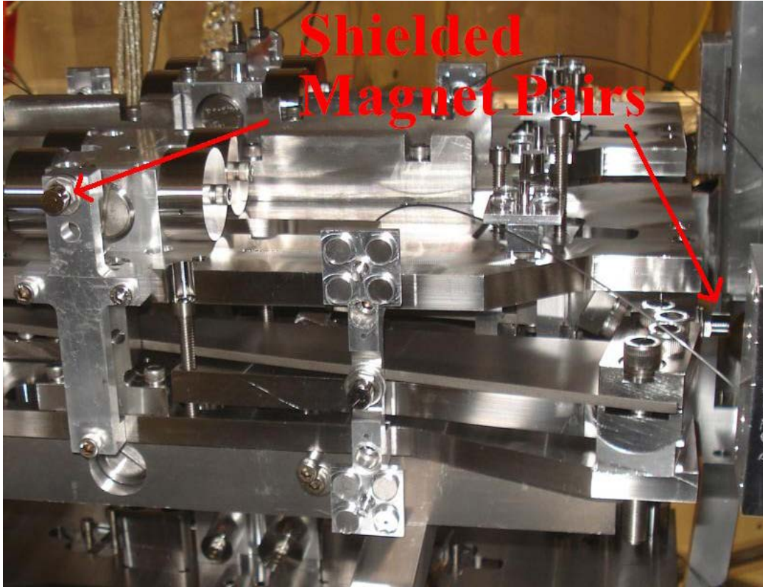
Figure 12 This photograph shows the locations of the shielded magnet pairs around the top mass. In LASTI notation these are the magnets belonging to the 'Side' and 'Face 1' OSEMs. The UI mass OSEMs also have shielded magnet pairs.
