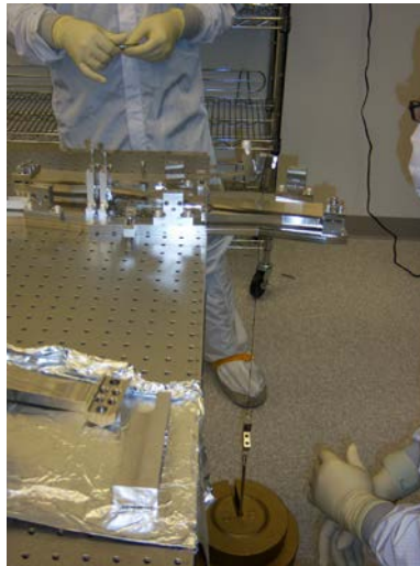
Figure 6 UI Mass with hanging weight to pull blade flat
