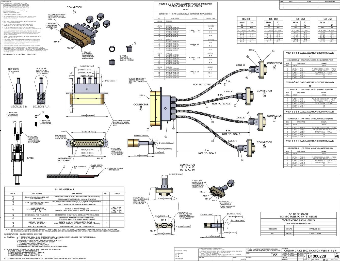
0228-v8 cable V25N8\_5\_8\_5, PART PDM REV., DRAWING
