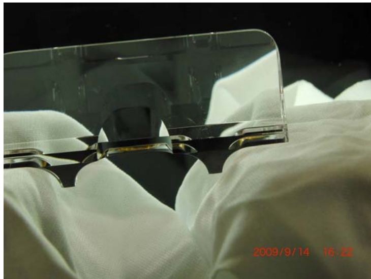
Unbonded, fully machined and polished ear between two crossed-polarizers
