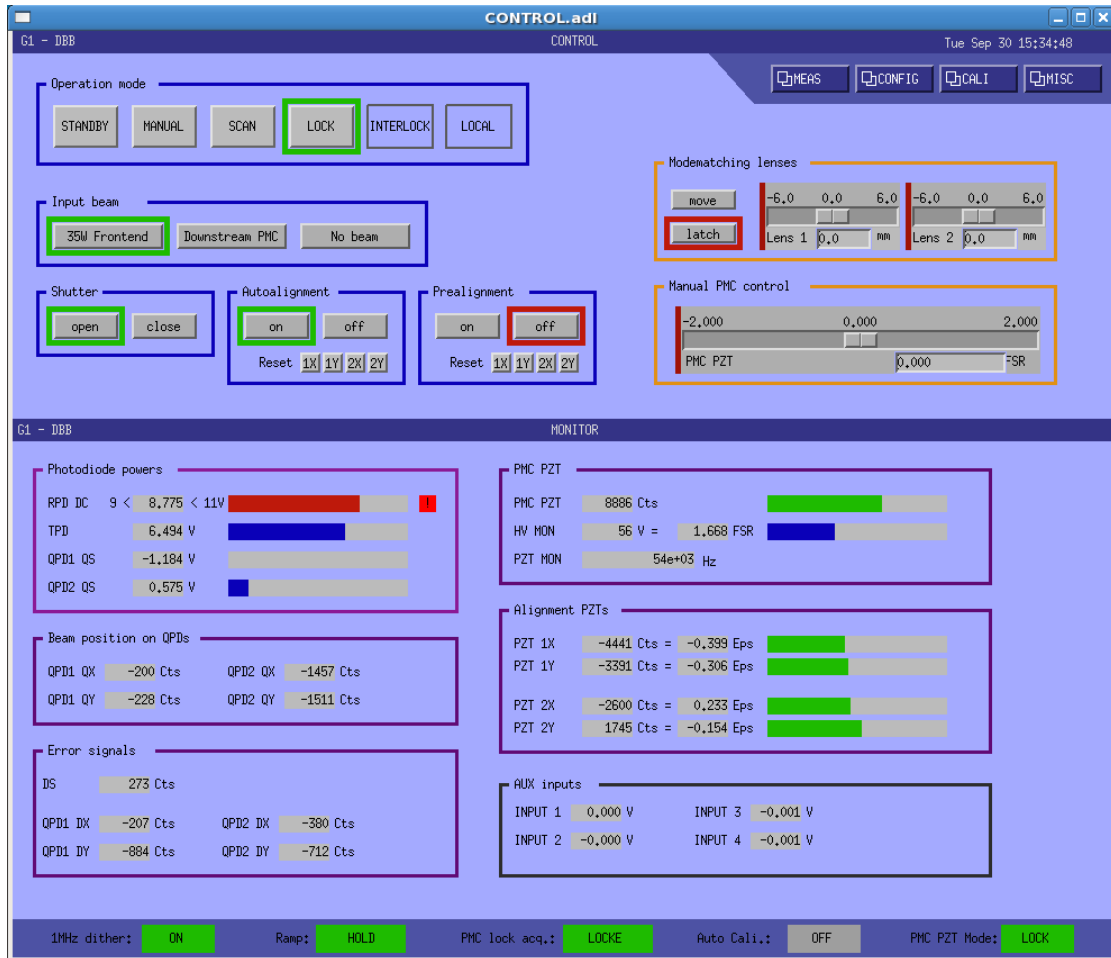
Figure 15: Main control screen for the DBB.
