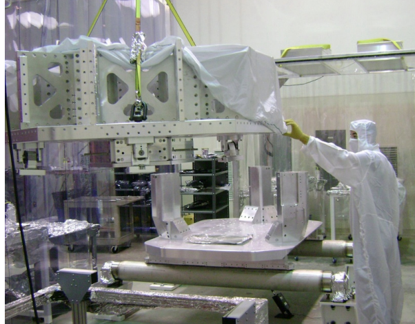
Figure 7. Jeff Kissel guides the partially assembled stage 1 structure onto stage 0. The three large vertical spring posts can be seen on stage 0.
