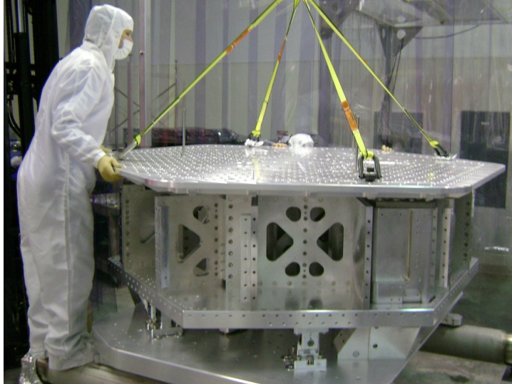
Figure 9. The optical table is guided into place as the top of stage 1.
