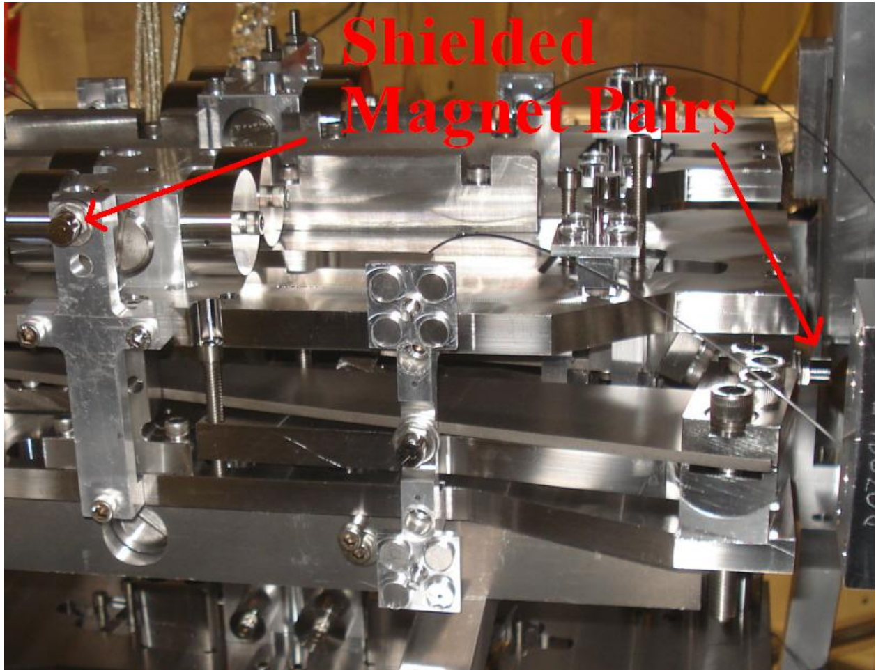
Figure 5: This photograph shows the locations of the shielded magnet pairs around the top mass. In LASTI notation these are the magnets belonging to the 'Side' and 'Face 1' OSEMs. The UI mass OSEMs also have shielded magnet pairs.
