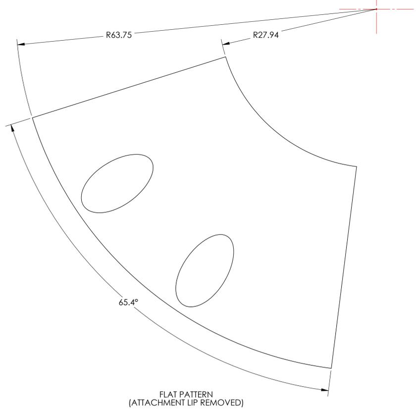
THIS PIECE IS PART OF A WELDMENT. DIMENSIONS SHOWN ARE APPROXIMATE; WELD INDUCED SHRINKAGE OR FILL, AND POST WELD ANNEALING AND MACHINING CONSIDERATIONS ARE NOT INCLUDED. SEE D0902654 FOR REQUIRED DIMENSIONS FOR STRUCTURE AFTER WELDMENT.
