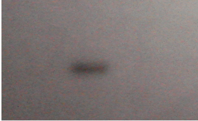
FIG. 25: Visible damage on SiC with 200\ \mu\text{m} spot size and 80 W power.
