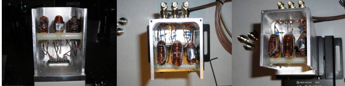
Figure 10: Resonant circuits with aluminum strips used to tune the resonant frequencies.
