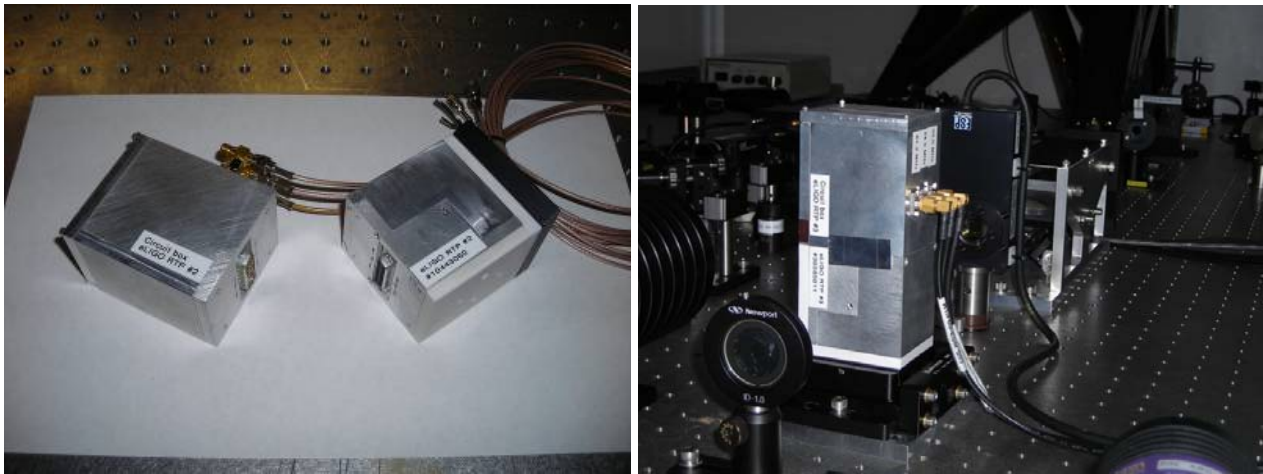
Figure 3 (left): Separate crystal and electronics box; (right) Modulator on LHO PSL table.
