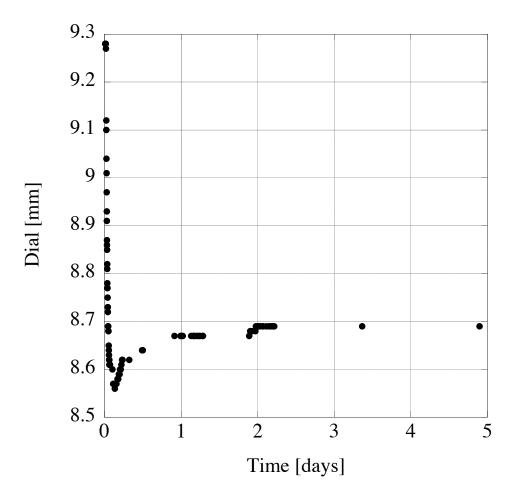
Figure 3: Creep behavior observed at 90°C. The initial creep, masked by the droop caused by the thermal variations of Young's modulus, is missed in this measurement.
