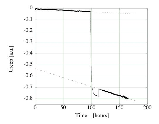
Figure 10: Exponential and logarithmic fit to a thermal transient data set.
