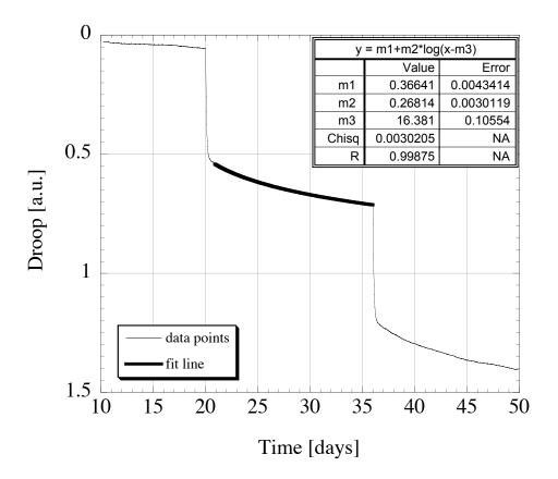
Figure 9. Creep slope evaluation for a blade, before and after a 10°C temperature raise. The linear fit before hour 98.4 and after hour 120 gave slopes of 0.00026 and 0.0016 respectively. The slope ratio of 6.11, from the fits in this figure, is the highest measured over the 6 blade measurements available. One of the DAQ jumps that eventually corrupted the long-term measurement is visible at about hour 115.
