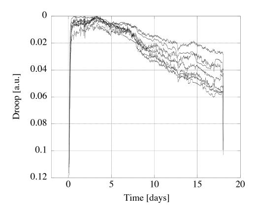
Figure 12: Correction force necessary to maintain the GAS spring at its working point as temperature changes.
