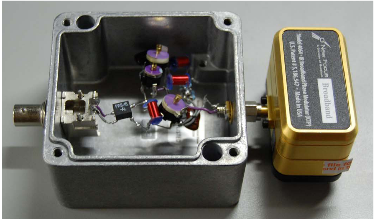
Figure 9: Picture of flying-component circuit in box attached to EOM
