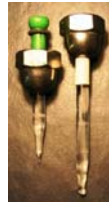
Fig 2. These ball shaped rods enable us to mount the fibres on a tensile testing machine.
