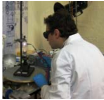
Fig 1. The fibres were pulled and welded to ball shaped rods (Fig. 2) using a H 2 -O 2 burner.
