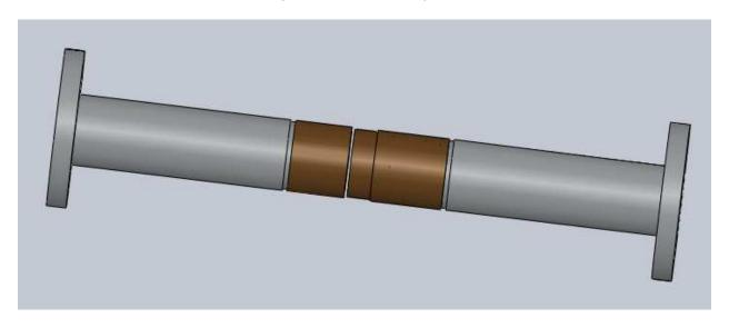
16. Set the quartz into the quartz holder and secure it with the cap. Lubricate the threads with IPA before tightening.
