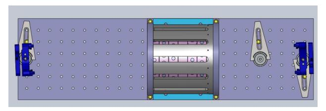
19. Attach the CWP assemblies to these two Siskiyou mounts with two #8-32x3/8" set screws. Make sure that the thick sides of the wedges are oriented as shown in the figure below.
