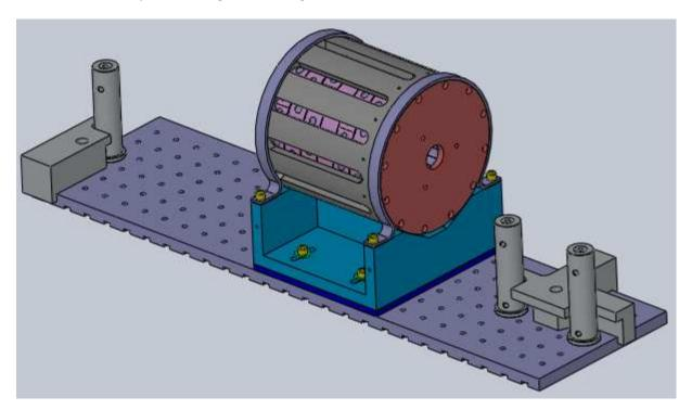
6. Get three forks and three  $\frac{4}{20x5}$  screws and use the forks to clamp the posts to the breadboard. Remove the alignment fixtures when finished.
