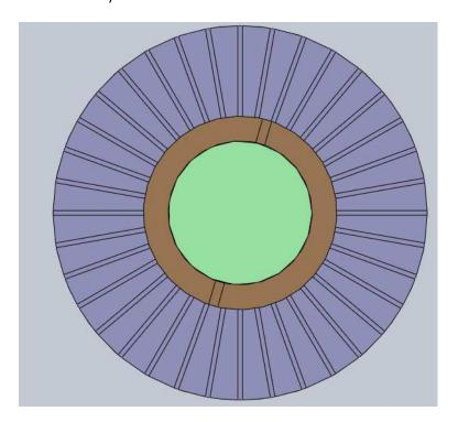
14. Assemble the TGG holders. Cut strips of indium foil that match the width and circumference of the TGG crystals. Roll a strip around each of the two TGG crystals and carefully slide the crystals into the TGG holders. You may have to gently bend the tines of the holder outward (by a very small amount) to get the TGG and indium to fit.
