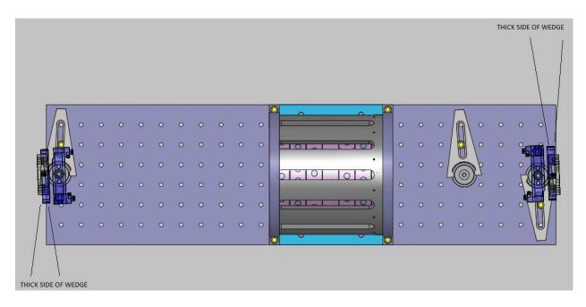
20. Follow the alignment procedures to align the CWPs and the TGGs and quartz rotator. The figure below shows the orientation of the TGG and quartz holders.
