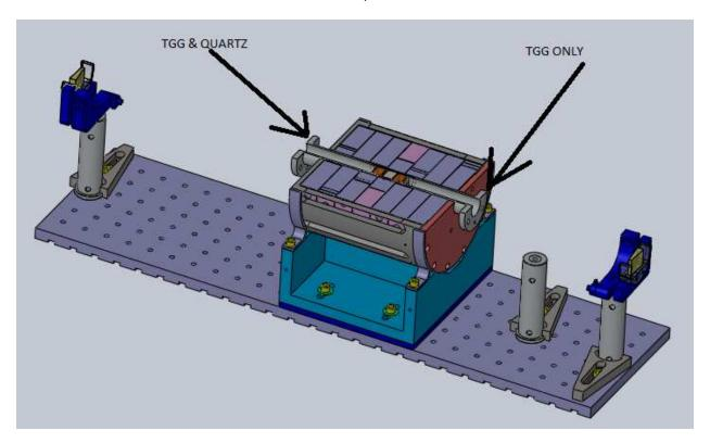
21. When the TGG locations are set for proper beam rotation, lock them into place with the positioning screws, threaded rods, sleeve lock, and hex nuts as shown below. Be sure that the tapped hole for the heat sink is at the bottom of both holders.
