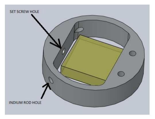
8. Insert the indium rod in the side until it goes a few mm past the set screw hole. If it bends under its weight slide it through so it is supported on both ends. Lift the calcite slightly so that it is centered in the mount and tighten the set screw.
