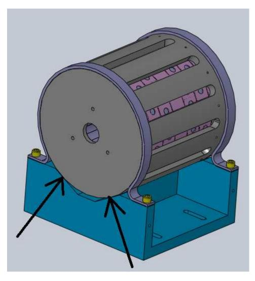
2. Get the spacer plate (pictured) and the breadboard to assemble with the magnet assembly.
