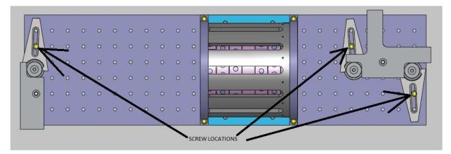
7. Assemble the calcite mounts. Set one piece of calcite on a clean-room cloth and set the CWP mount over it. The mount has a threaded hole at the top for a #8-32x3/8" set screw, and a hole in the side for inserting the indium rod.
