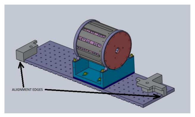
5. Take three of the posts with the engraving "L1 HAM2 FI 3.735" and set them on the breadboard so that they are flush against the alignment fixtures.
