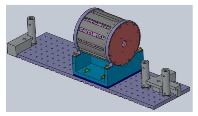
6. Get three forks and three ¼-20x5/8" screws and use the forks to clamp the posts to the breadboard. Remove the alignment fixtures when finished.
