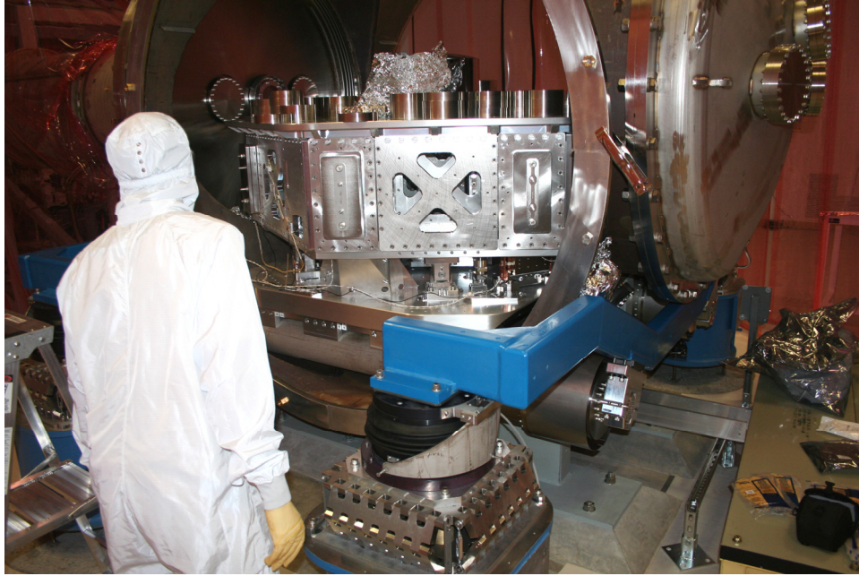
Figure 2. The HAM ISI installed in its chamber at LHO.
