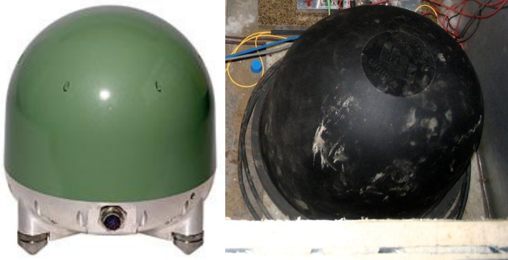
Figure 44,45: Trillium 240 (left) and the same seismometer installed with its protective and insulating rubber cover (right)
