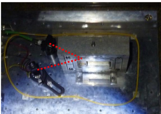
Figure 50,51: the optical lever used in the horizontal seismometer prototype is shown on the left, the dotted red line denotes the optical path from laser transmitter reflecting to the PSD (4) . In the right the laser emission spectrum
