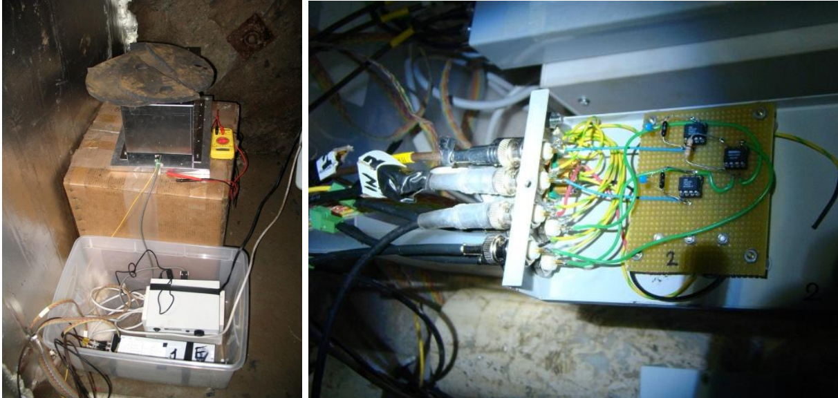
Figure 52,53: on the right the laser source is shown in the metal box, while the laser power supply, DC power supply and electronics boxes are in the plastic box; on the left an electronic box opened during the work
