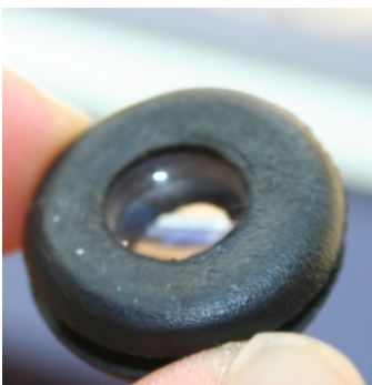
Figure 4: Beam expander lens mounted in rubber grommet
