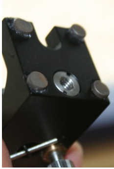
Figure 2: Permanent magnets glued to the base of an OptiSigma Mirror mount
