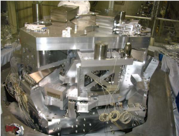
BSC-ISI as built for the prototype installed at LASTI
