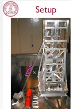
Damping strut setup & Result on the Tech Demo at Stanford
