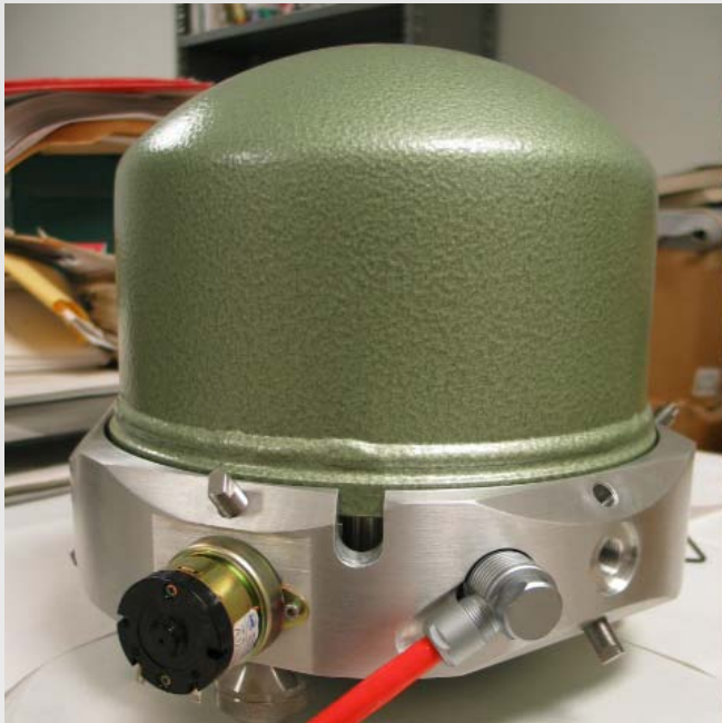
STS-2 Diameter: 9.5 in Dia. with lockerMtrs: 13.5in Height: 9.5 in Weight: 21 lb
