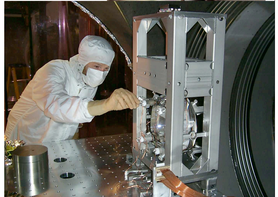
Optics suspended as simple pendulums on 0.25 mm wire
