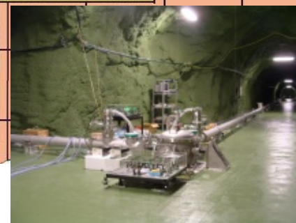
Laser strainmeter with 100-m arms
