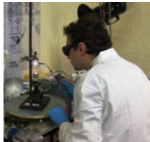
Fig 1. The fibres were pulled and welded to the ball shaped rods using a H 2 -O 2 burner.
