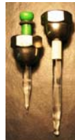
Fig 2. The ball shaped rods enable us to mount the fibres on a strength test machines.
