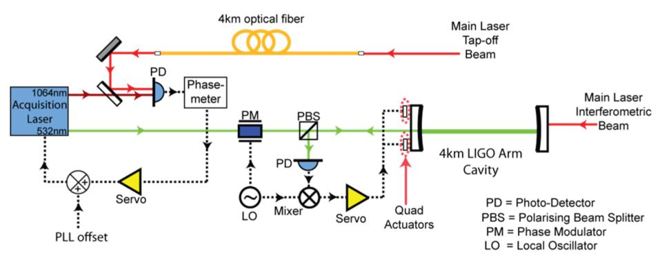
Step 5: Hand-off the feedback to the quad actuators, to lock the cavity length to the frequency of the laser.
