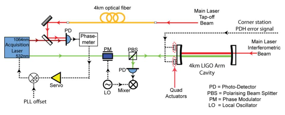
Step 8: Finally, switch feedback from the Acquisition Laser to the Main Laser.
