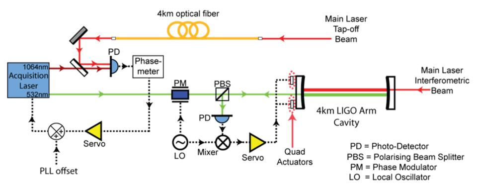
Step 7: Tune PLL offset to bring cavity onto resonance with the main laser
