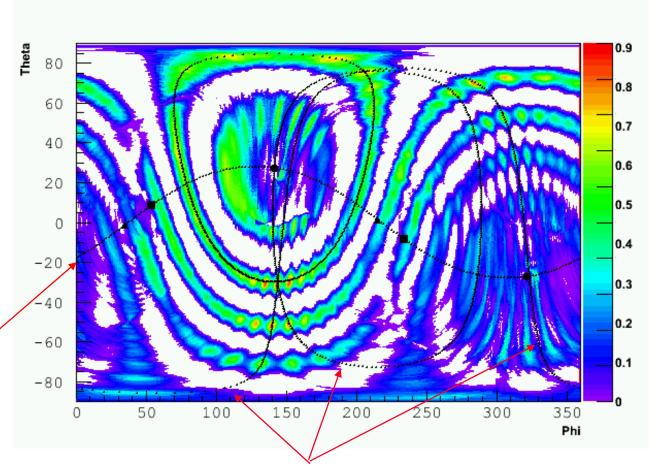
constant delay rings for detector pairs
