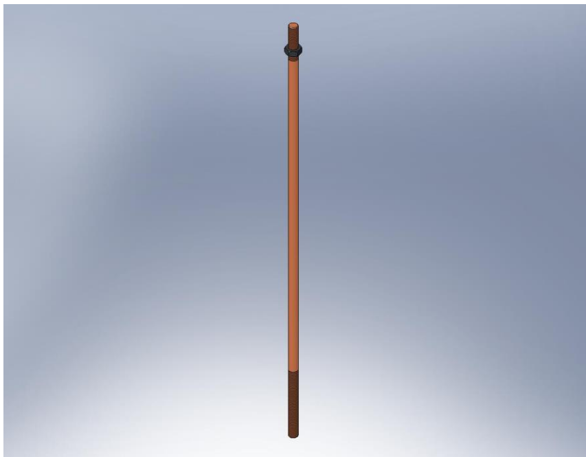
Figure 4.63. Thread the jam nut onto the end of the Pull Rod with 2" of thread.
