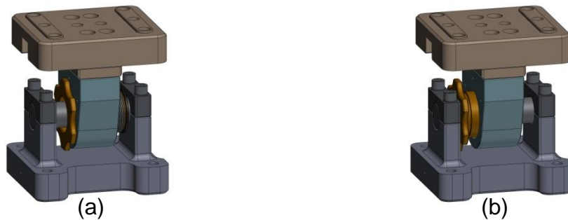
Figure 3.18. Locker Assembly in (a) “unlocked” and (b) “locked” positions. To lock the assembly, turn the knob end of the Locker Sleeve counterclockwise, until the retaining ring contacts the back face of the Locker Housing. Note: the Assembly still slides freely when in the locked position.
