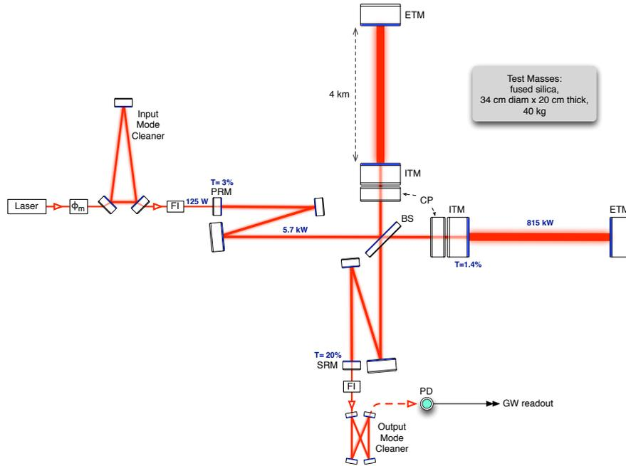
Figure 1: Interferometer layout with stable recycling cavities; both recycling cavity beam paths are folded within the mode cleaner tubes, between HAMs 2 and 3 for the PRC and between HAMs 4 and 5 for the SRC.
