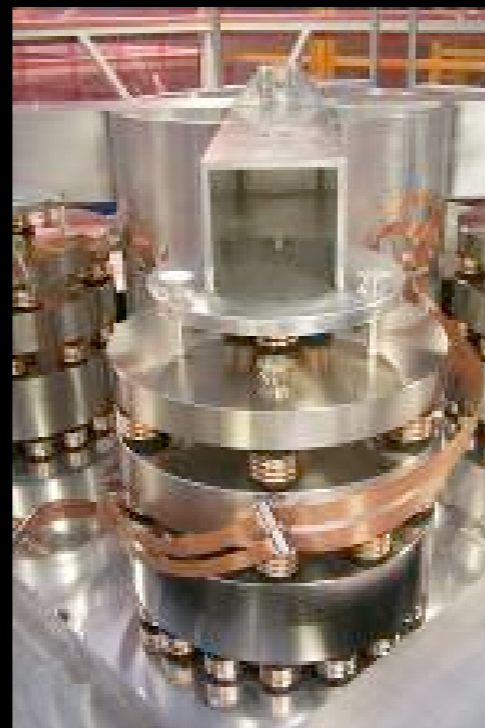
Seismic Isolation Stack
