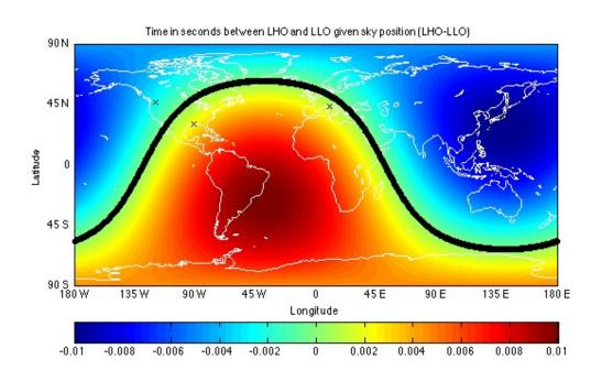
A ring of sky locations is constrained using the detection delay between the 2 LIGO detectors.
