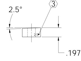
DIMENSIONS ARE IN INCHES NAME CALIFORNIA INSTITUTE OF TECHNOLOGY MASSACHUSETTS INSTITUTE OF TECHNOLOGY CIT/RJ 05/02 TOLERANCES: .XX ±0.01 CHECKED **ADVANCED LIGO** .XXX ±0.005 SUB-SYSTEM SUS ANGULAR±.25° LIBRARY OF CLAMPS PART NAME LOWER BLADE CLAMP LOWER SIDE ANGLED (2.5°) 302, 304 OR 316 SSTL COMMENTS: SIZE DWG. NO. REV. D020336 SCALE: NTS
