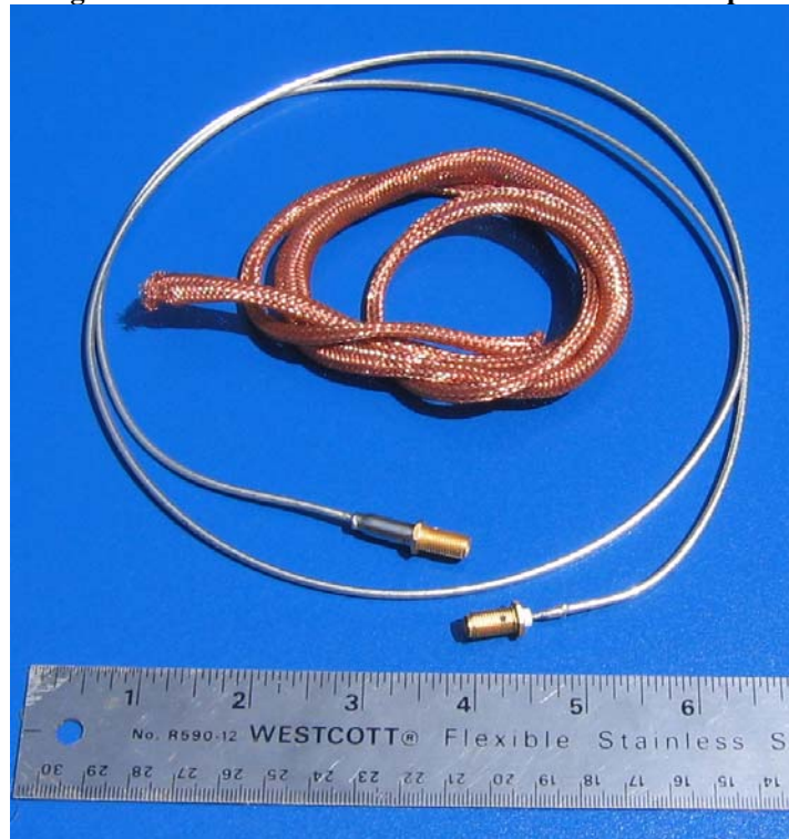
Figure 5 LIGO Braid and Reference Belden 1671 Sample
