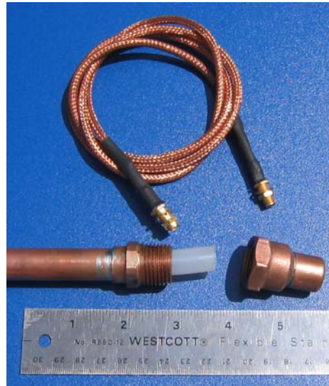
Figure 3 Removable End of Triaxial Test Fixture and Braided LIGO Cable Sample
