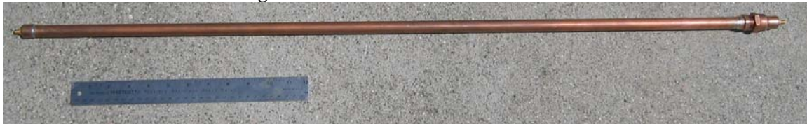
Figure 2 One Meter Triaxial Test Fixture
