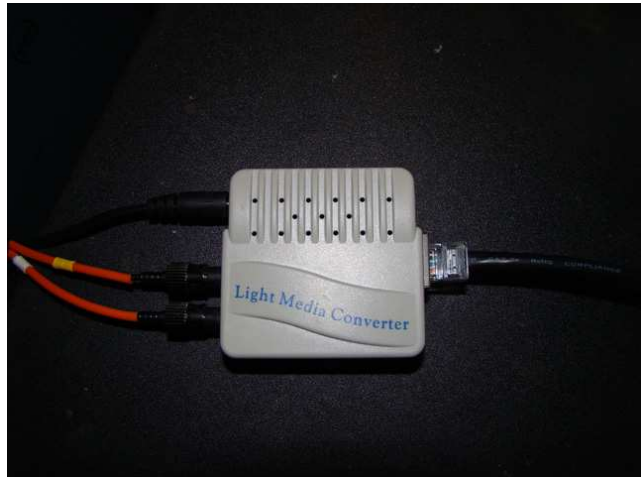
Figure 19: Light Media Converter. It converts duplex ST into RJ45 (standard copper-ethernet connectors). A pair of transceivers is specified to transmit data over distances up to 2 km with 100Mbit/s.
